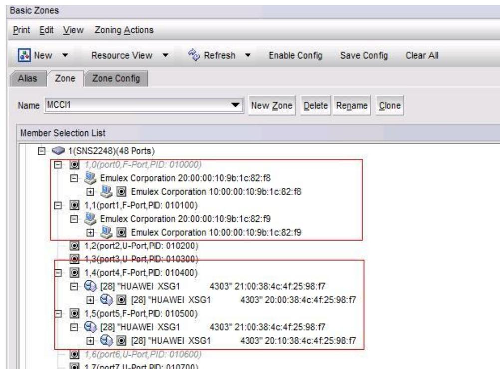
In this example, the hosts use ports 0 and 1, while the storage systems use ports 4 and 5. The display indicates that the switch has correctly identified the devices connected by the four ports.
