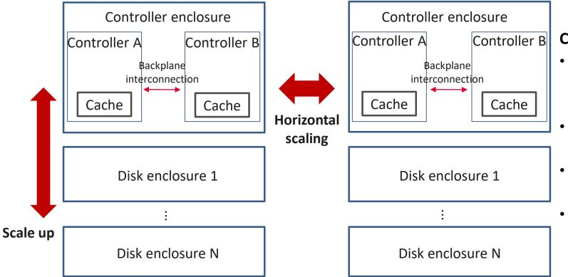
Note: Devices that support multiple controllers can be expanded horizontally. Generally, a maximum of 32 controllers are supported.
