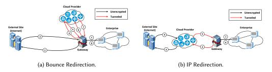
Fig. 6. Middleboxes virtualization with NFV and SDN [38].
