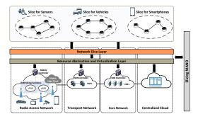
Fig. 12. Conceptual illustration of network slicing.
