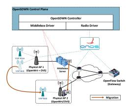
Fig. 10. NFV/SDN architecture for WiFi networks.
