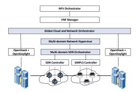
Fig. 13. An NFV/SDN architecture design for SDN-enabled VTNs [81].
