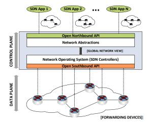
Fig. 2. SDN Reference Architecture [4, 5, 14].
