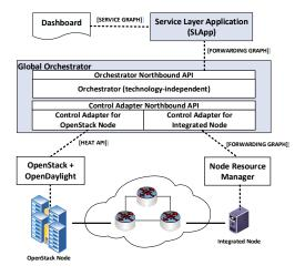
Fig. 9. An NFV/SDN architecture design for vCPE.
