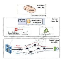
Fig. 5. NFV/SDN architecture for application-specific traffic steering.
