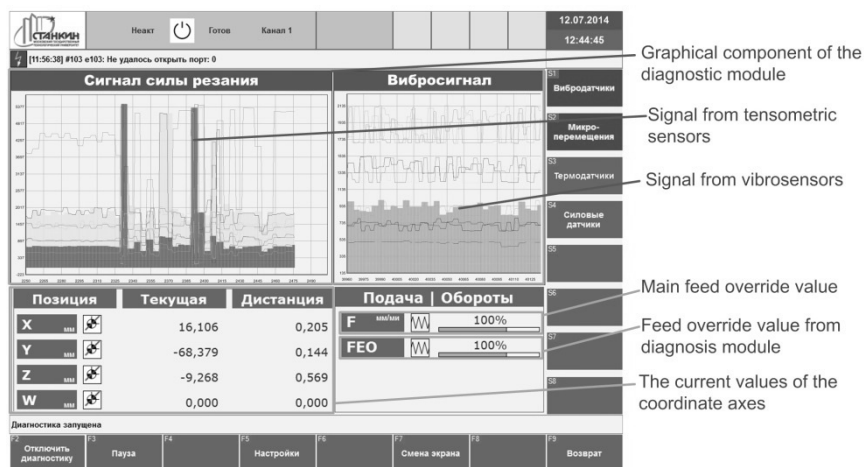
Fig. 8. The interface of terminal part of the diagnostic mode in the CNC system
