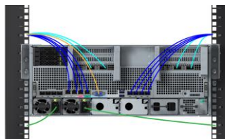
OceanStor Pacific 9546(1机箱1节点, 每节点2 CPU)线缆布放规则
