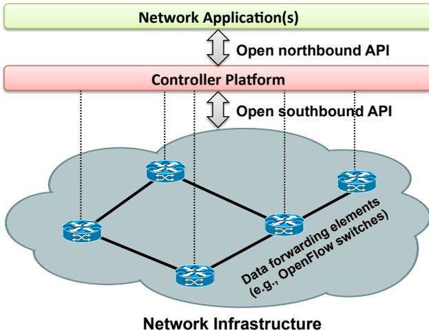
Fig. 1. Simplified view of an SDN architecture.
