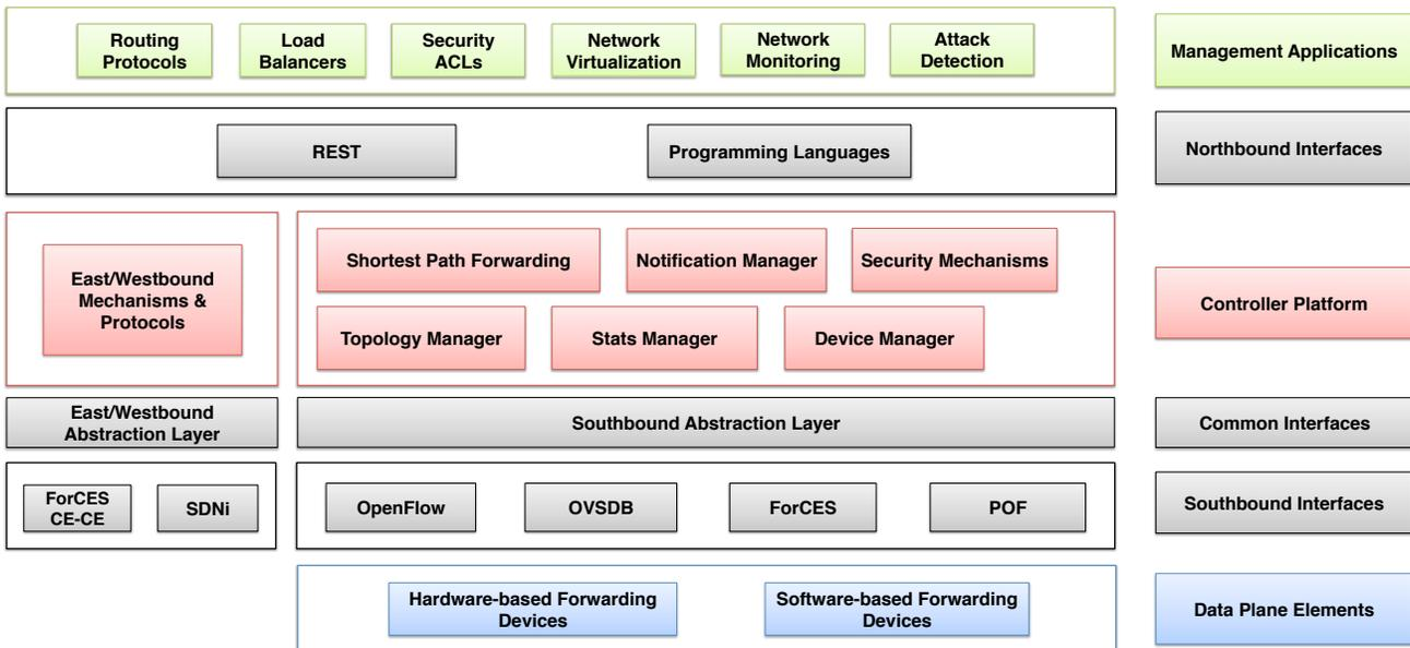
Fig. 8. SDN control platforms: elements, services and interfaces
